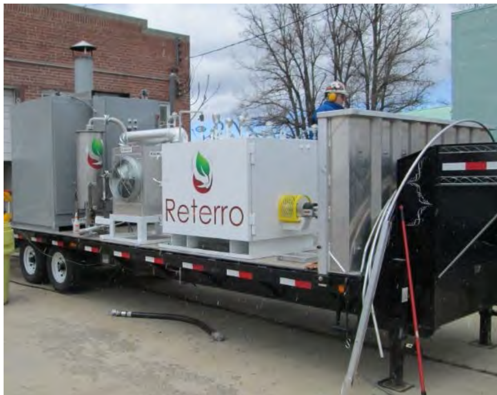
Reterro Mobile EDU with Thermal Oxidizer
